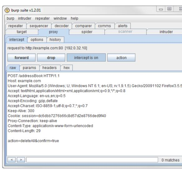
This screen shot of the Burp proxy shows an example of a request vulnerable to CSRF. All of the parameters to the application (*action, confirm*) are predictable.
