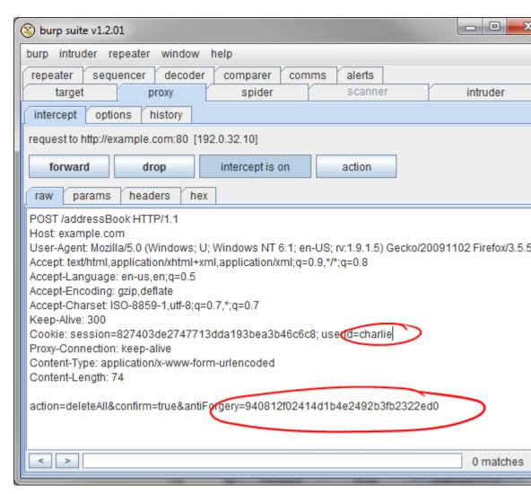
This application global anti-forgery token could be observed by one user and used to attack other users.
