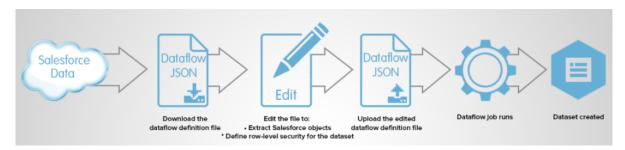
To configure the dataflow, you add transformations to the dataflow definition file. A *dataflow definition file* is a JSON file that contains transformations that represent the dataflow logic. You can add transformations to determine what data to extract, how to transform datasets, and which datasets to register to make available for queries.
