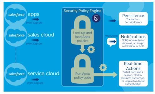
The Transaction Security architecture uses the Security Policy Engine to analyze events and determine the necessary actions.
