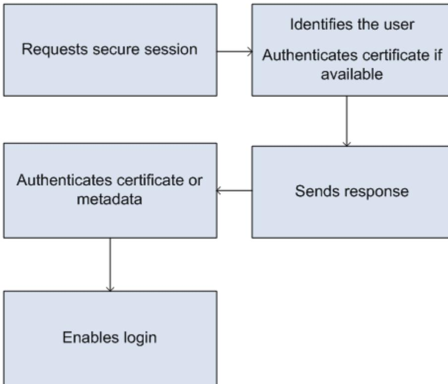
1. The service provider sends a valid SAML request. The endpoint is automatically generated when the service provider is defined—the SP-Initiated POST Endpoint.
