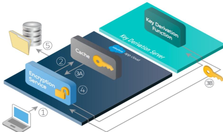
1. 1. When a Salesforce user saves encrypted data, the runtime engine determines from metadata whether the field, file, or attachment should be encrypted before storing it in the database.
